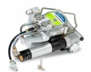
The PHT1402 is a heavy-duty pneumatic strapping tool that delivers a secure friction weld seal on flat and round surfaces. Perfect for larger duty securement jobs, the PHT1401 pulls up to 1,280 pounds of tension and is easy to handle.
