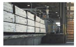
Polyester (PET) it the strapping of choice for pressure treated wood thanks to its elongation and recovery characteristics. Loads of lumber are unitized before treatment. The PET strap does not corrode from the treatment chemicals unlike steel strapping that can rust and stain the wood.
