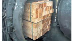
Here, the lumber emerges from pressure treatment. PET strapping has the strength of steel strapping but unlike steel, it has elastic properties to stretch and hold the expanding package secure without cutting into and deforming the wood. Straps stay tight and absorb impacts without breaking.
