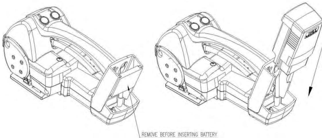
**E - SAFETY INSTRUCTIONS :** To start working, remove the spacer and insert the battery until the safety button clicks as shown in picture
