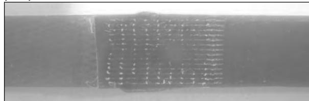
NO – seal strength insufficient
