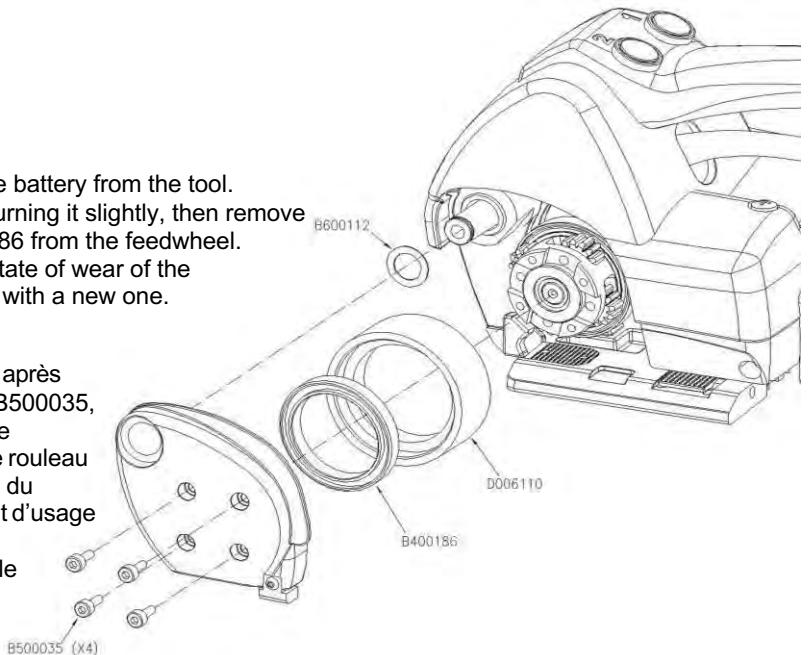
**E** - To replace or clean the feedwheel first of all remove the battery from the tool.
