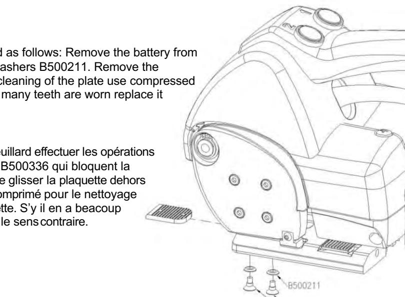
**E** - For cleaning or replacement of the strap locker proceed as follows: Remove the battery from the unit, remove the 2 screws B500336 and remove the 2 washers B500211. Remove the straplocker from the front using a pliers with long jaws. For cleaning of the plate use compressed air. Check the state of wear of the teeth and then replace, if many teeth are worn replace it with a new one. To replace run in reverse order.
