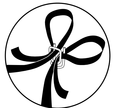
How to Thread Cord Strapping onto Metal Buckles
