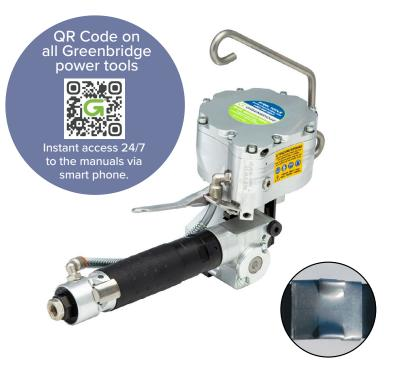
SP4000 Series Steel strapping tool for 1/2", 5/8" or 3/4"(13, 16 or 19mm) steel. Tensions and seals on steel strap up to .031" thick. Pulls tension up to 1,700 lbs. Tool weighs approximately 8.5 lbs. Utilizes push type seals and produces a single notch joint.
