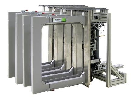
The MHB is a custom built side seal strapping machine designed to strap product vertically. The unique head location is designed to minimize foreign matter from interrupting machine performance. Designing a multiple head system can dramatically increase your production. Constructed with heavy-duty material and hardware allows this machine to operate flawlessly in virtually any environment.
