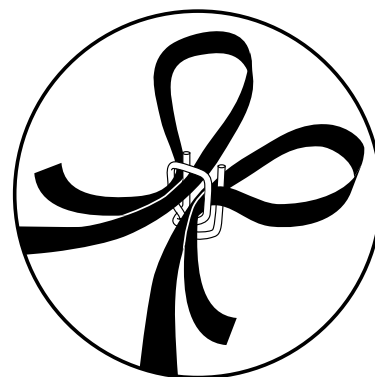
How to Thread Cord Strapping onto Metal Buckles
